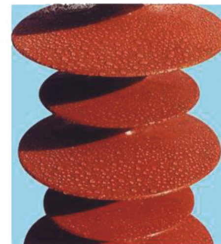
Enhancing methods of silicone rubber holds good hydrophobicity and anti-leakage current tracking capacity.
